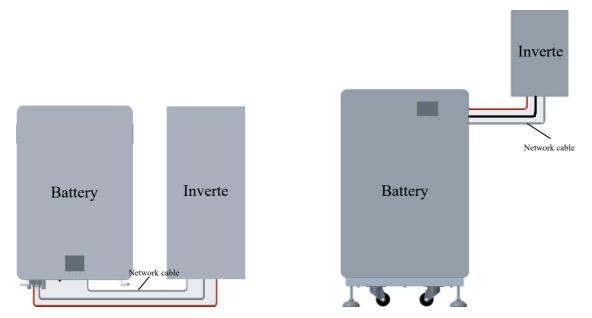
If a single battery is used, follow this step. If multiple batteries are used in parallel, set each battery's address code according to Table 3.4, and connect the RJ-45 to RS485 communications ports in sequence. Connect the RS485 port on the first or last battery module to the BMS communication port on the inverter.
